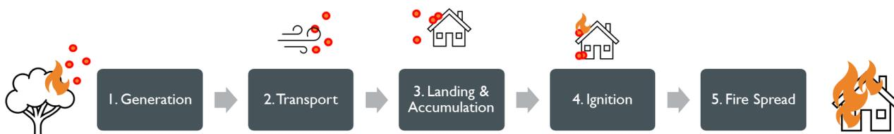
Figure 1: Schematic diagram of the five subprocesses of wildfire firebrand building ignition and damage: 1) firebrand generation, 2) wind-driven transport, 3) landing and accumulation, 4) building ignition and 5) fire spread.
