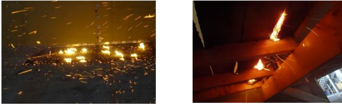
Figure 2. Top of deck (left) and under-deck (right) views of ignited decks during the ignition potential series of experiments. Table 1 tabulates a summary of all the ember exposure tests.
