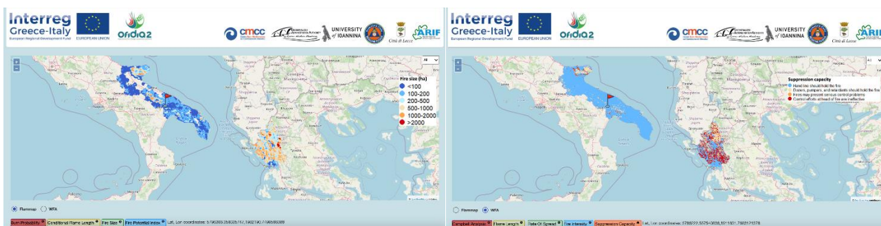
Figure 5 – Examples of the fire behaviour modelling outputs showed by the web GIS of the OFIDIA2 DSS. On the left, fire size calculated by FlamMap; on the right, suppression capacity calculated by WFA.
