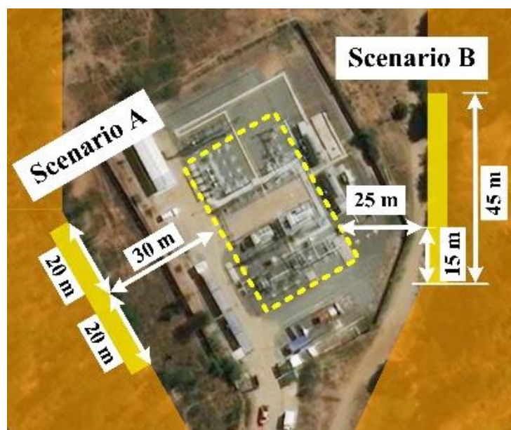
Figure 10- Scenarios for estimating incident heat flux on a target within the substation. Orange indicates a wildfire engulfing the substation perimeter; yellow rectangles represent the flame fronts considered.
