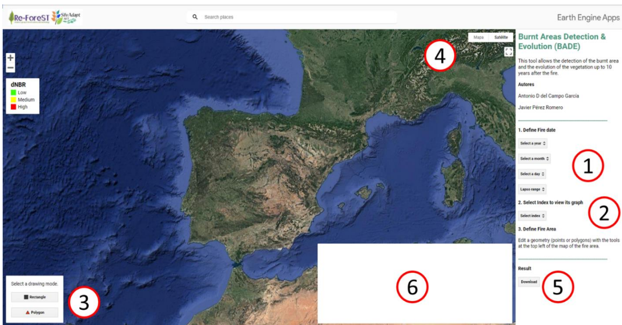
Figure 2: Parts of the graphical interface of the BADE tool. 1. fire dates; 2. selected index for the time series; 3. draw region of interest where the fire occurred; 4. layers visible on the map; 5. download image of fire severity classes; 6. time series graph of the selected index.
