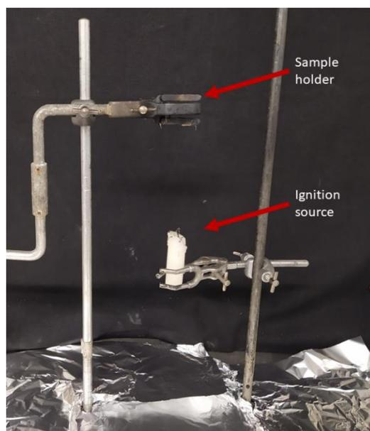
**Figure 4. The Molinia grass ignition testing apparatus**
