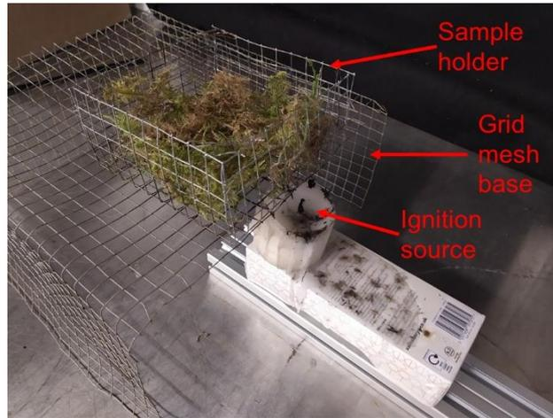
Figure 5. The moss testing apparatus: sample holder, base mesh grid, and ignition source are indicated.
