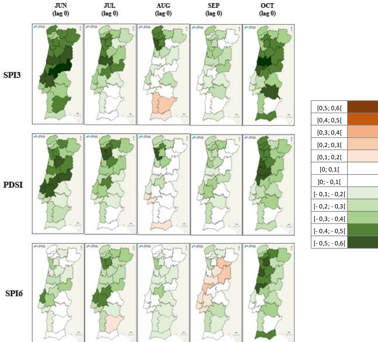
Figure 3 - Correlation coefficient between monthly forest fire occurrences and monthly SPI3 (upper row), PDSI (middle row) and SPI6 (lower row) drought indices from June (on the left) to October (on the right) at a NUT III level. Negative correlation in greenish shades and positive correlation in brownish shades.
