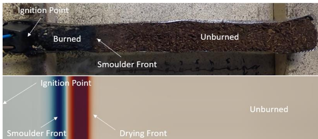
Figure 3- Top: Lateral peat spread experiment, smouldering direction left to right; Bottom: simulated peat smouldering, where red represents the drying front and blue represents the pyrolyzing front
