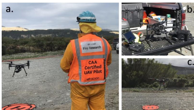
Figure 1. Pilot taking off Matrice 210 with DJI XT2 camera prior to burn commencing; b. Setting up Matrice 210 UAV; c. DJI Matrice 600 craft taking off, carrying MiniVUX lidar sensor as payload.
