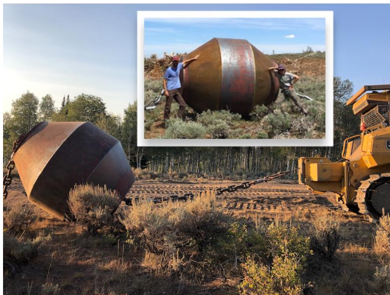
Fig. 1. Roller-felling barrel situated centrally between two cables and dragged between a pair of bulldozers. The cable fells trees, while the large barrel drum keeps the cable roughly >1m above the ground surface, providing necessary leverage to pull over trees. Once felled, variable amounts of slash can be retained, while remaining debris is pushed into a pile and burned at a later time. Inset photo for scale.
