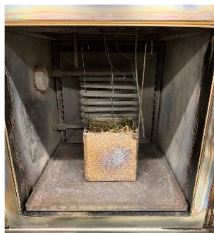
Figure 5 – SEDEX-Oven with 100g soil sample
