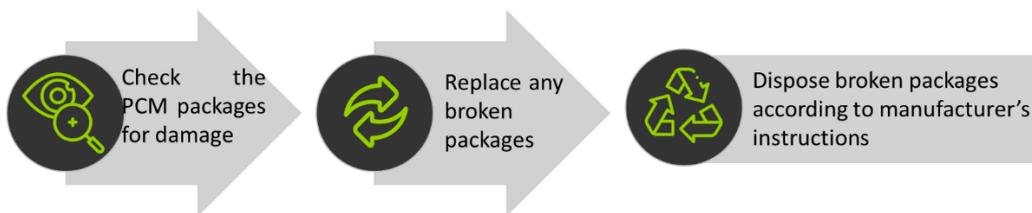
Figure 3. Inspection and disposable procedure for PCM packages
