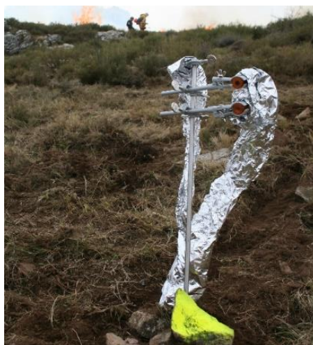
Figure 3- Radiant and total heat flux sensors and thermocouple fixed on supporting rod and protected by aluminum foils.
