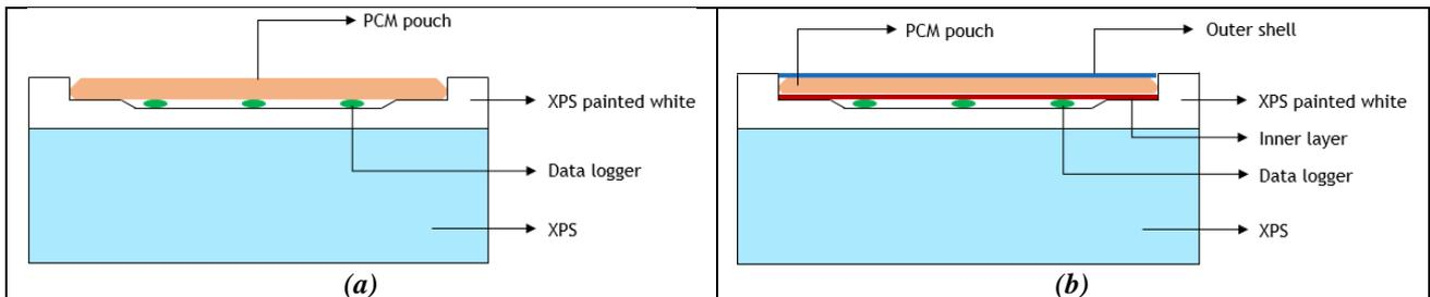
**Figure 2 - Schematic representation of the experimental set-up for the transient behavior evaluation tests considering: (a) only the PCM pouch and (b) the assembly outer layer + PCM pouch + inner layer.**
