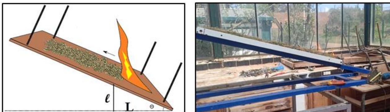
Figure 3- Inclined fire propagation table.
