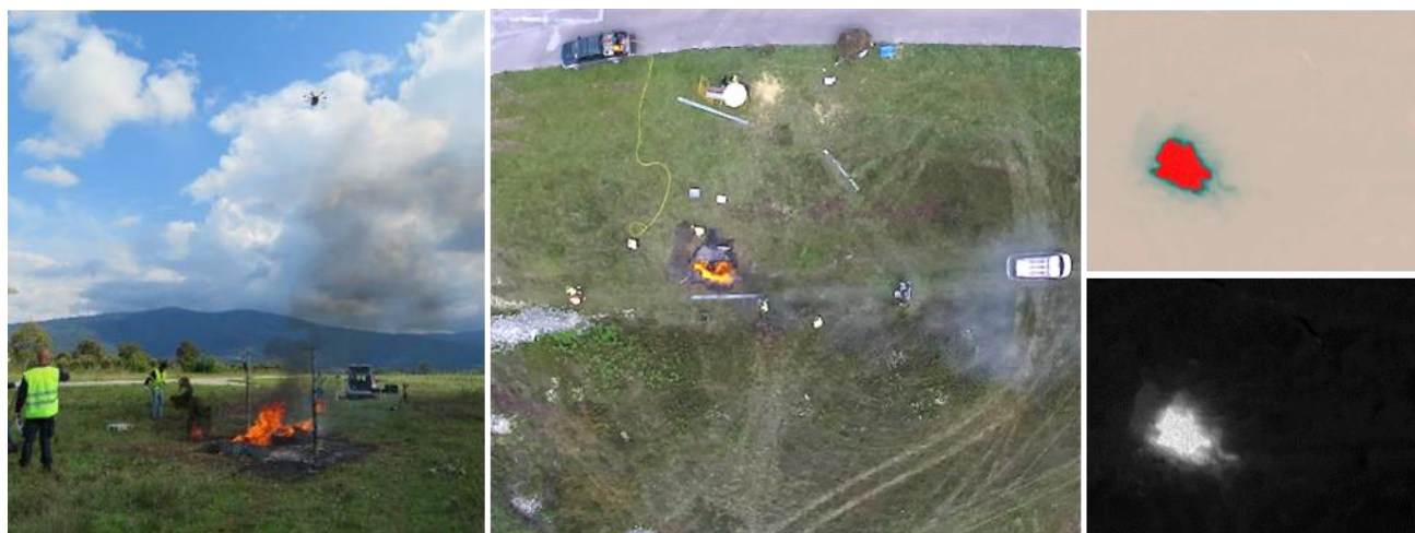
Figure 4 – Examples of aerial images captured in the tests. Left: Tests setup; Middle: Visible range image in RGB color space. Top-Right: Thermal image processed with a linear automatic gain control algorithm, encoded with the GrayRed color palette. Bottom-Right: Thermal image processed with a plateau equalization automatic gain control algorithm, encoded with the Grayscale color palette.
