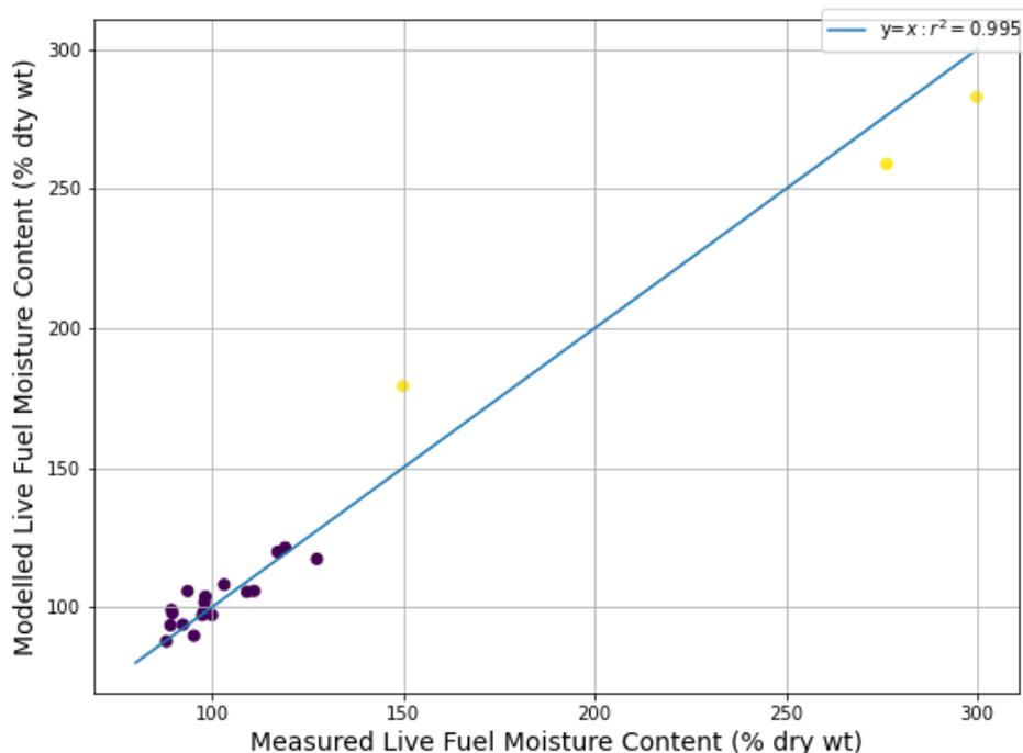
Figure 4 – Preliminary model predictions of live fuel moisture as a function of specific leaf area, relative water content and surface-area-to-volume ratio using a fixed  $k$  parameter for new and old foliage.
