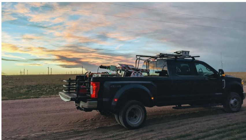
Figure 2- Doppler lidar and scanner installed in the bed of an F-350 pickup truck.
