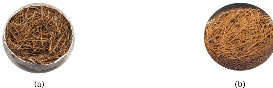
Figure 2 - Fuel samples for the tests with (a) buoyancy-induced flow using the basket of 0% opening and (b) forced flow using the basket of 63% opening.
