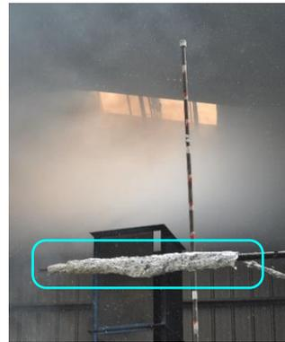
Figure 4. S-type pitot tube in the experiments.
