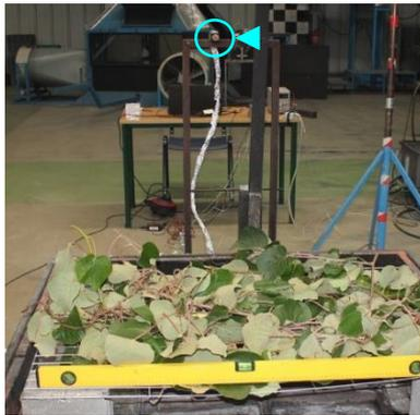
Figure 3. The location of the heat flux sensor.
