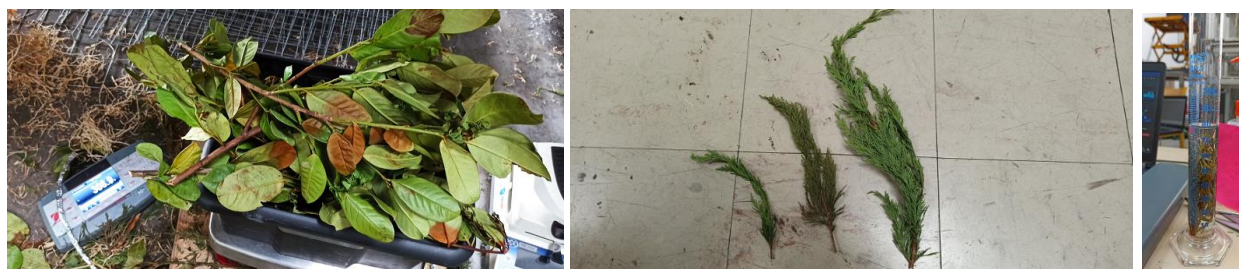
Figure 5 – Property measurements: (left) oleander weighting, (middle) cypress branches clustering for size distribution evaluation, (right) cypress bulk density evaluation
