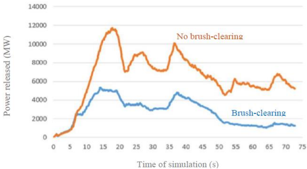
Figure 4 - Temporal evolution of the power released by the fire in the entire simulation domain (« Château C1 ») according to the fuel treatment.
